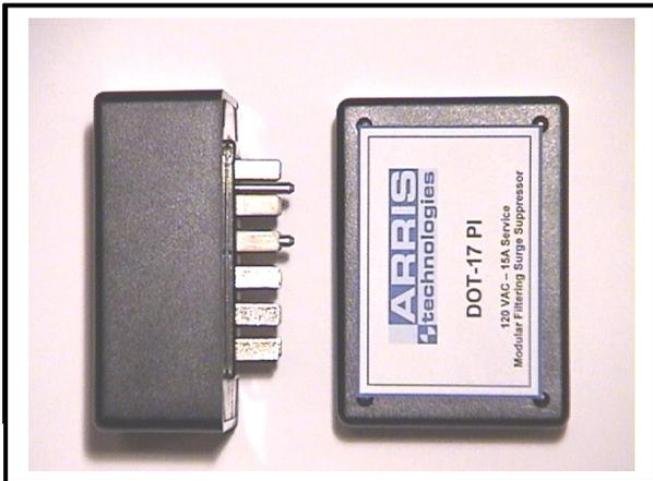
The **DOT-PI** is a modular Series Hybrid surge suppressor and EMI/RFI line filter intended for ITS traffic cabinet applications. The **DOT-PI** incorporates multiple metal oxide varistor (MOV) surge suppression stages along with a series line LC Pi filter stage to provide clean, lightning protected power in a compact modular plug-in unit. The active components are epoxy encapsulated in a rugged, high temperature phenolic case for safe and reliable operation.
